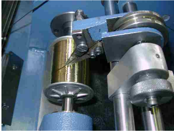
Beak type wire guide for winding spring steel wire
